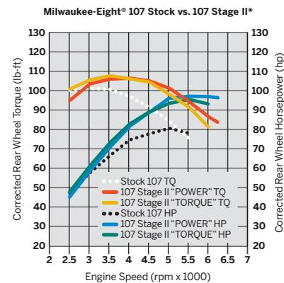
\* FLHX 107 Stage II "POWER" with Ventilator A/C & Street Cannon Mufflers
