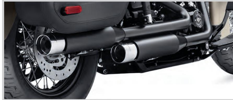
**C. SATIN BLACK MUFFLER SHIELDS – SHORT (SHOWN ON FLHC MODEL WITH SATIN BLACK EXHAUST SHIELDS)**
