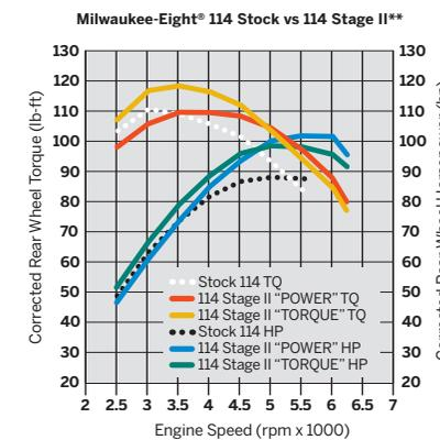
\*\* FLHXSE 114 Stage II "POWER" with Ventilator A/C & Street Cannon Mufflers
