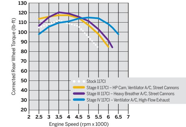
DYNAMOMETER (DYNO) PERFORMANCE TESTING: Declared performance values in this catalog represent SAE J-1349 transient peak power output. Dynamometer settings, motorcycle condition, variation, climate and other factors can affect performance output and results can vary from the performance values declared by Harley-Davidson.
