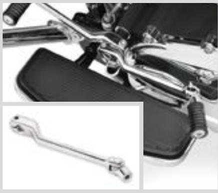
**F. KLAPPBARER FERSENHEBEL – EINGEKLAHPTE POSITION**
